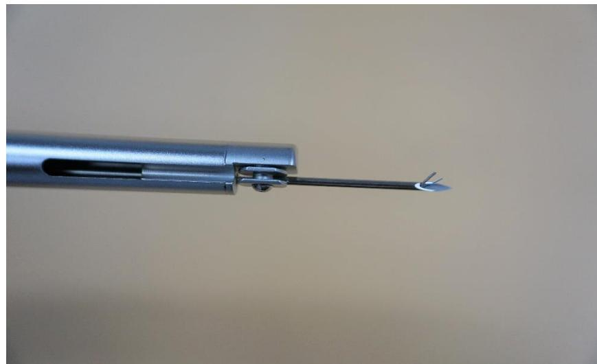
7. Verify that only the electrode stimulating tip of the electrode is exiting the needle tip of the Disposable Electrode Delivery Tool.
