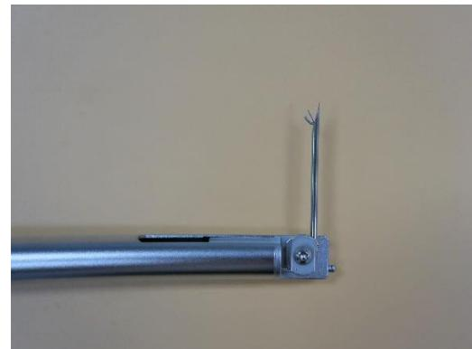
9. Verify that only the electrode stimulating tip of the electrode is exiting the needle tip of the Disposable Electrode Delivery Tool.
