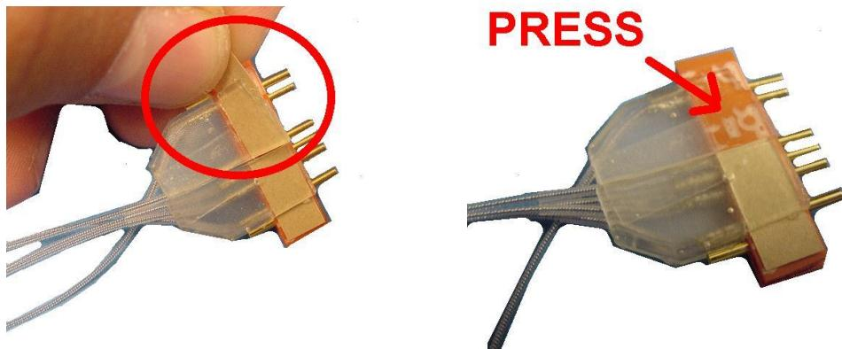
6. Remove the adhesive liner on the right side and press firmly on the connector as shown.
