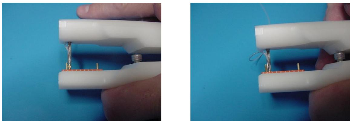
10. Select the next cephalad electrode and insert into the 5<sup>th</sup> hole in the electrode connector.
